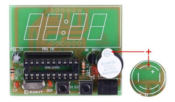
Step 7: Install 1pcs 4Bit Red Clock Digital Tube at DS1 and pay attention to its installation direction. Note that the four decimal points are below.
